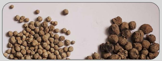
**Sintagg** sintered flyash lightweight aggregates is made from the sintering process of fly ash as per <u>IS CODE 9142 PART 2</u>. Sintagg is formed into small round pellets, which are then processed to creates a very hard aggregates with a honeycombed internal spongy structure. These hard pellets can then be used as a superior, consistent, lightweight aggregate which is up to 50% lighter than natural aggregate.
