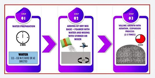
LITAGG CELLKON developed with LC3 (Lime Calcined Clay Cement) Technology
